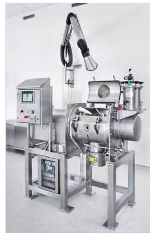
Lödige Ploughshare<sup>®</sup> Mixer type FKM for batch operation for small production and laboratory purpose
