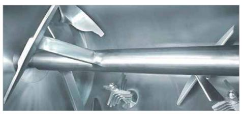
Fully welded mixing elements in hygienic design
