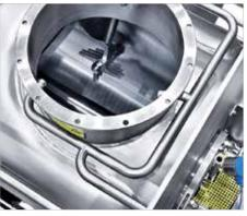
Cleaning nozzles for WIP cleaning process
